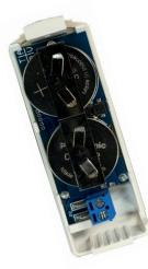
The Door/Window Sensor with Extended Contact is a supervised, wireless sensor that detects the opening and closing of doors or windows.
