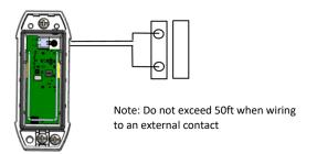
Note: Only one set of contacts can be used at one time the internal or external, for added security the internal reed switch can be cut.
